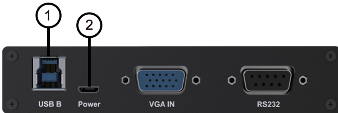
Figure 10. Rear USB ports for powering up an elinkKVM device
